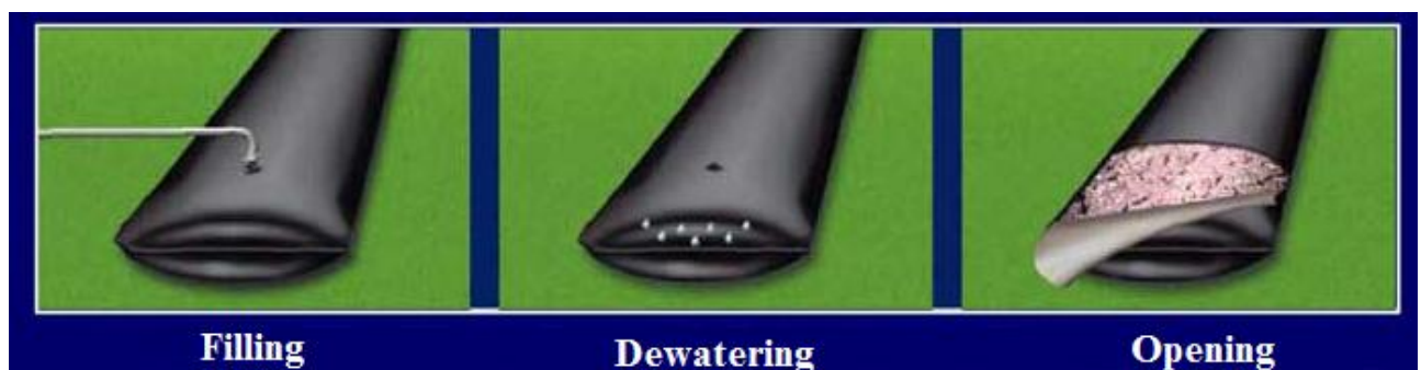
Figure 11. The principle of sludge dewatering in geotextile bags
