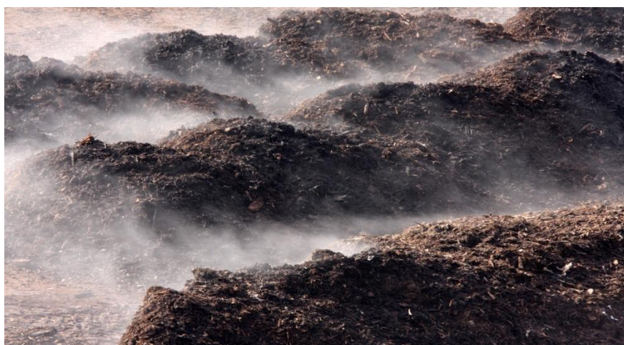
Figure 26. Composting of sewage sludge
